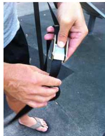
Figure 6. Depress the “Press” portion of the buckle to allow the webbing to feed through & adjust the length of the webbing.
